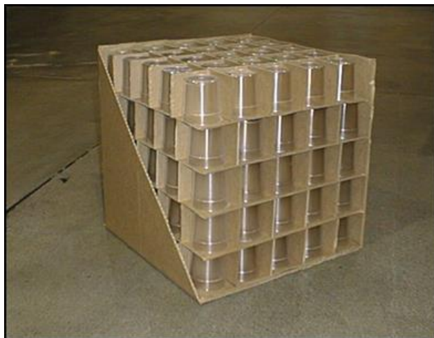
Figure 35 – Cut away of single box showing cups.
