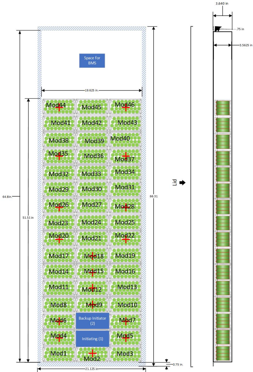
Figure 191 – Initiating unit instrumentation layout.
