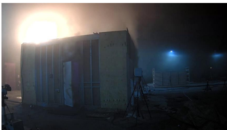
Figure 154 – Conditions at test termination (54 minutes) in Test 4.
