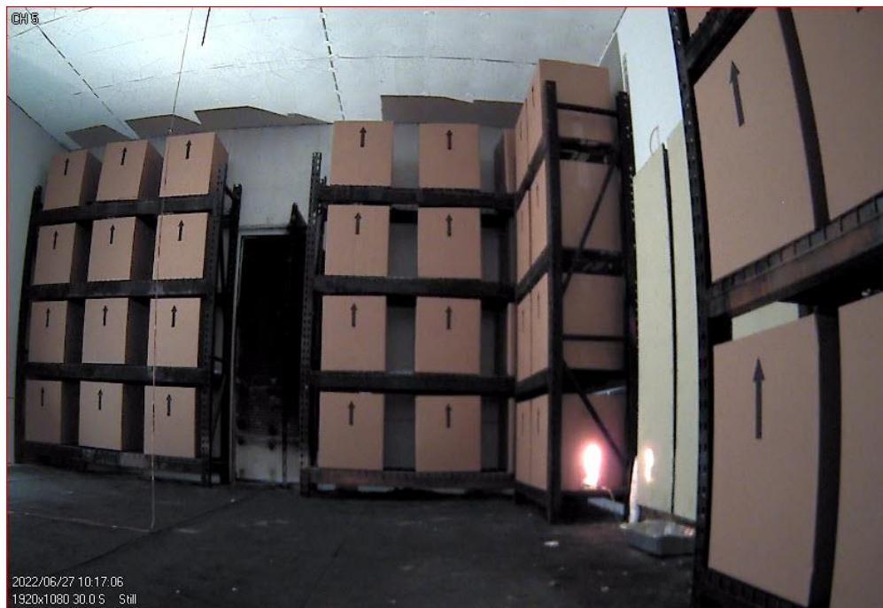
Figure 119 – Ignition of Group A commodity using an electric match at time 00:01.
