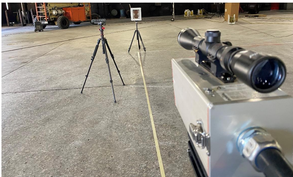
Figure 50 – Example of tunable diode laser emitter and reflector.
