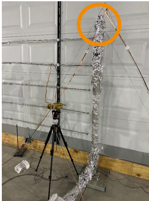
Figure 47 – Heat flux gauge placement (outlined in orange).
