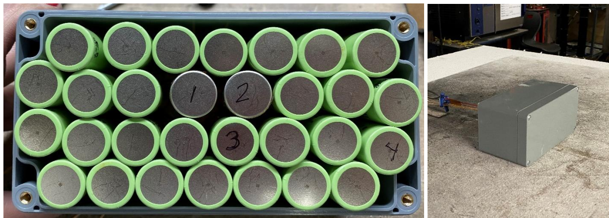
Figure 187 – Module construction (left) and assembly (right).
