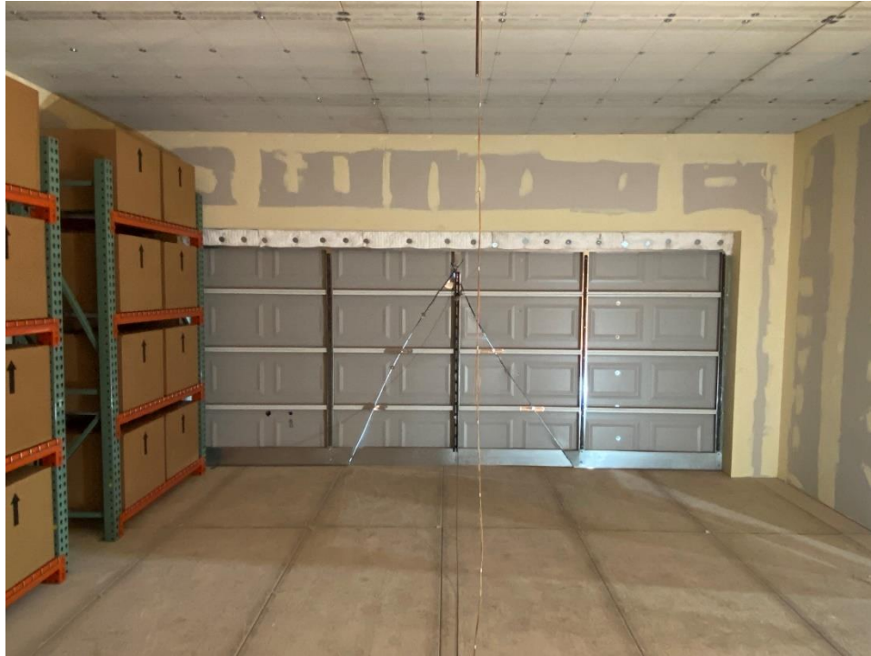
Figure 30 – Test structure (Garage door interior).
