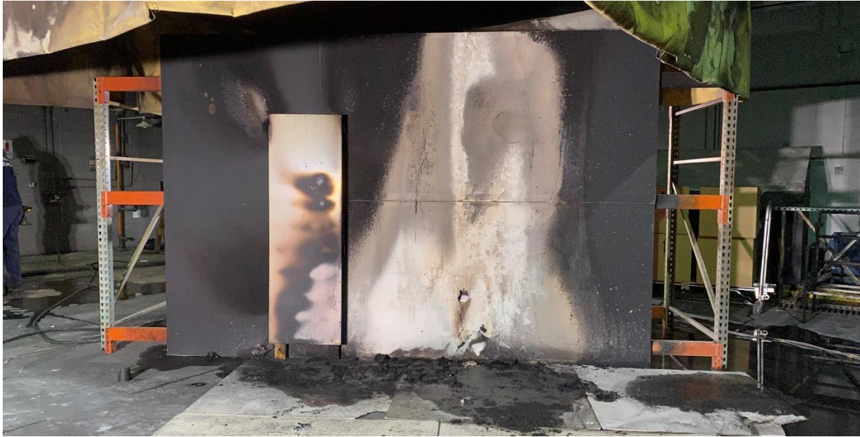
Figure 199 – Post-test condition of ESS unit and Commodity boxes in Scenario 2.
