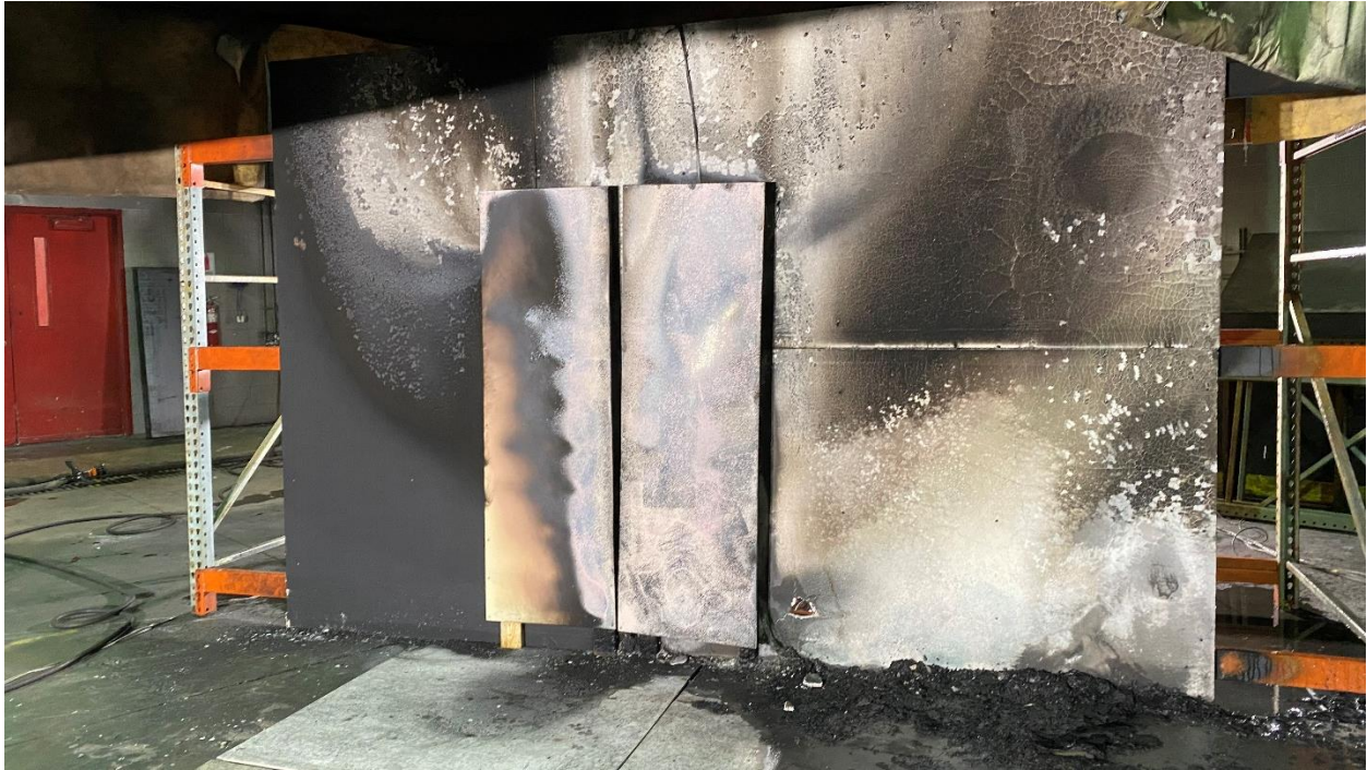
Figure 195 – Post-test condition of ESS units and Commodity boxes in Scenario 1.
