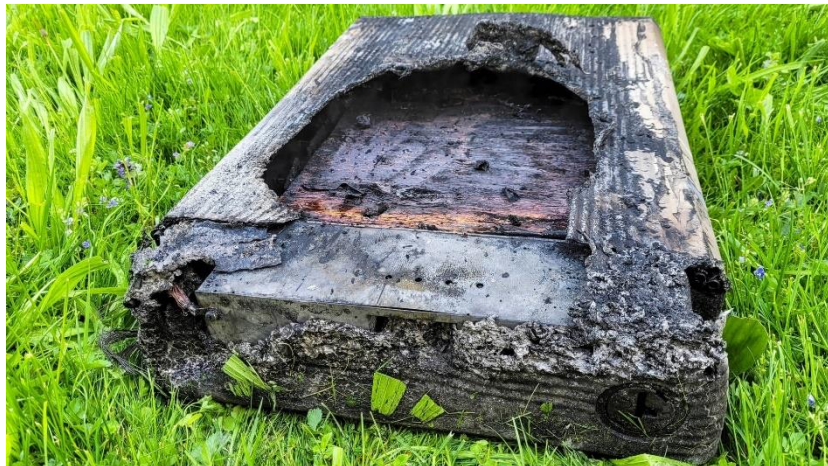
Figure 17 – Battery condition following incident [23].
