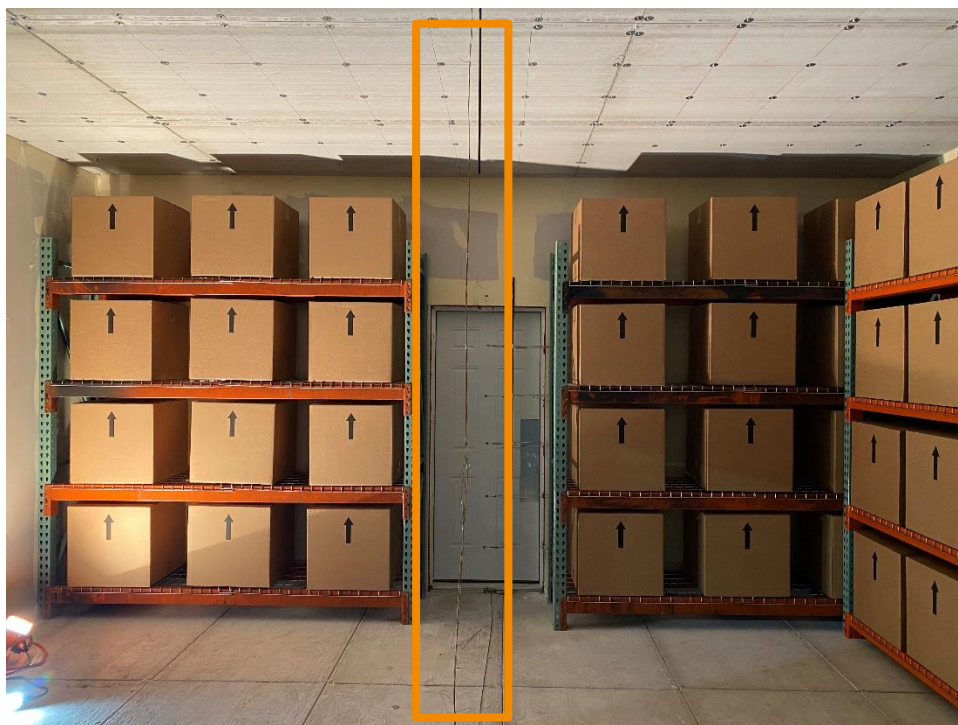
Figure 40 – Thermocouple array (outlined in orange).
